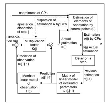
Figure 1. Block diagram of discrete nonstationary filter for estimating the elements of exterior orientation.
