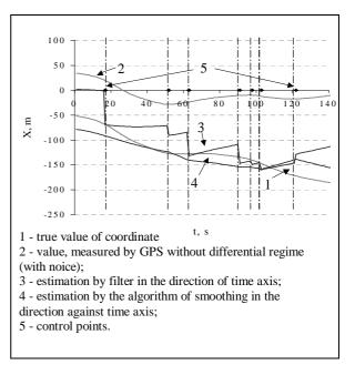
Figure 2. Example of the estimation of coordinate X.
